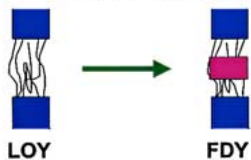
Figure 19 Intermediate layer scenario to explain the observed stiffer network behaviour of the FDY yarns.
